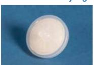
Designed for filtration and purification in a sterile environment. Fisherbrand™ Sterile PES Syringe Filter features a PES membrane in a polypropylene housing for purification of tissue culture solutions from a standard syringe. 33mm diameter membranes available with 0.2 or 0.45µm pore sizes.
