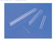
Use these tubes for cell washing procedures. Fisherbrand™ Borosilicate Glass Light-Walled Culture Tubes are made of borosilicate glass to reduce pH changes and contaminants potentially leached from soda lime glass.
