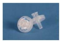
Designed for daily routine analysis. Fisherbrand™ Nonsterile PTFE Syringe Filter features a hydrophobic PTFE membrane for filtering HPLC organic solutions. Available in two membrane diameters (13 and 25mm) and two (0.2 and 0.45µm) pore sizes.
