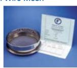
Made from stainless steel and available in a wide variety of sizes. Fisherbrand™ Stainless Steel Test Sieve with Woven Wire Mesh has a 200mm diameter.
