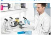
Perform sample transfers between virtually any tube, rack, microplate or horizontal gel box quickly and efficiently with adjustable tip spacing.
